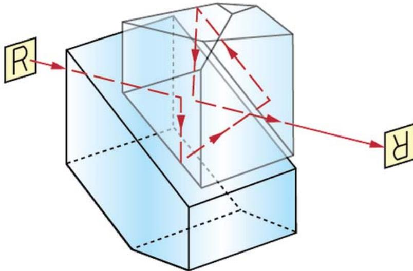
**Figure 5:**  $180^\circ$  Rotation with a Pechan-Roof Prism
