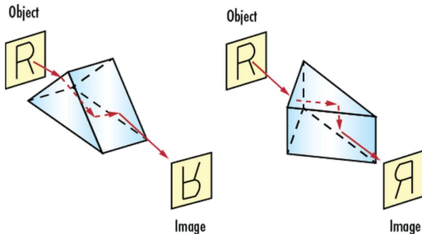
**Figure 3:** 180° Rotation with a Pechan-Roof Prism
