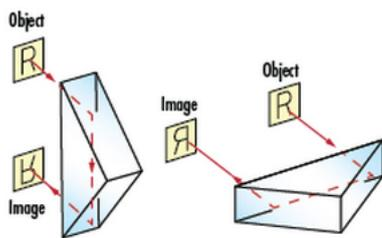
**Figure 2:** Fixed 180° Rotation with a Porro System
