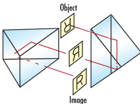
**Figure 4:** Fixed 180° Rotation with a Porro System
