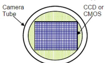
Face view of a Camera Pick-Up Tube Sensor, with a CCD superimposed on the imaging face, to illustrate the correlation of Format Types.
